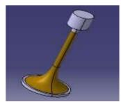
Fig. 4: Valve Specimen Stellite
